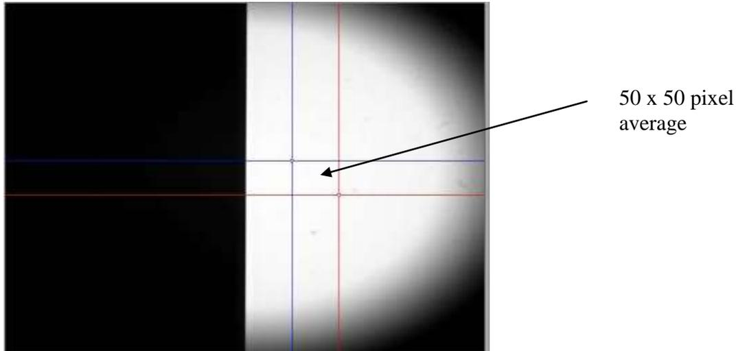
The dark noise can be calculated by taking the difference of image A-B. Finding the histogram of the differences and taking the square root of the sum of these variances in the area above will give the RMS noise. In this case, the noise is derived from the signal difference rather than the dark level. This is done to get around the black level clamp that mask the dark noise level, assuming the clamp can be turned off.
